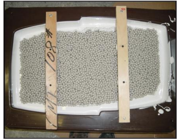
Figure 7. Syntactic is cast around and through core.
