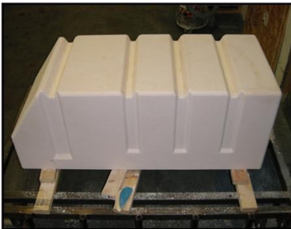
Figure 11. Syntactic foam plug for freezer liner.
